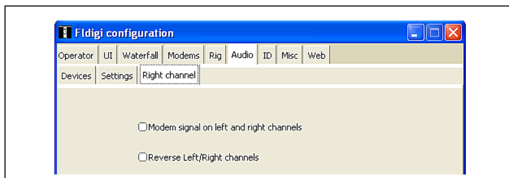
Figure 9: Default fldigi audio channels. No options are selected, which means that the Left audio channel is used for TX audio (and ignored by the TS-590S)
