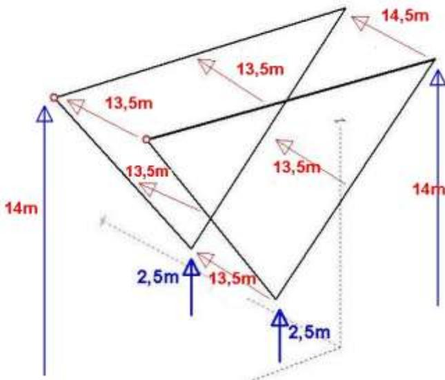
Currently my 'provisional' 80m antenna experiment consists of TWO Phased 'Inverted' DELTA LOOPS, VERTICAL polarisation. Average Elements distance is about 63 degree. The average Antenna height is 13-14 m.
