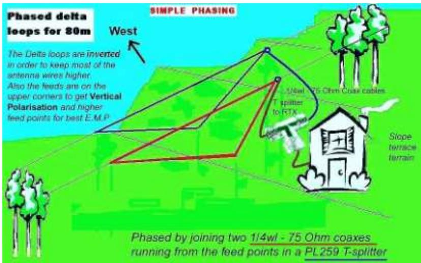
This system of BROADSIDE phasing is very simple and uses just two 1/4 wl 75 Ohm coaxes joined together (it is not actually a 'real' broadside because the loop antennas are clearly able to beam in 2 directions only that are perpendicular to the loop plane).
