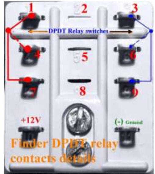
I am provisionally using three cheap **DPDT** (Double Pole, Double Throw) Relays of the brand **Finder 12V – 10A**, Teflon insulation.
