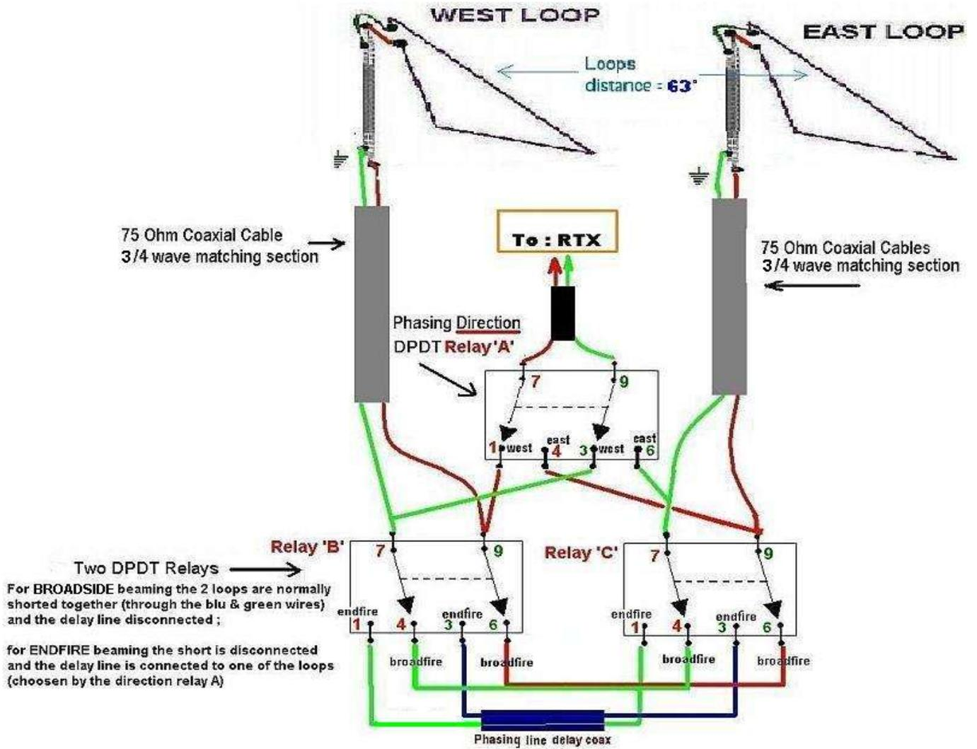
For **BROADSIDE** beaming the 2 loops are normally shorted together (through the blue & green wires) and the delay line is disconnected.
