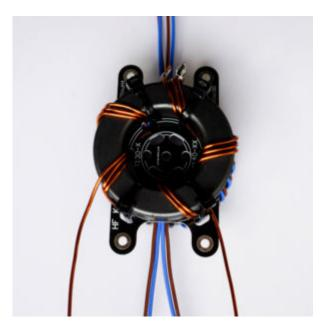
Now solder the BalUn and the impedance transformer together as shown in the picture below. Cut the wires as short as possible but so that they can still be soldered together.
