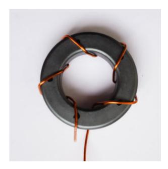
Now wrap another five windings (red) parallel to the first five with the same wire. Cut both wires. (length approximately 1.5 cm) Now scrape the ends of the winding wire bare with a sharp knife or sandpaper. This has to be done properly, otherwise soldering will be difficult.
