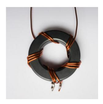
TIP: For a nice flat SWR curve over the entire frequency spectrum, it is important that the three windings run tightly against each other. Use small cable ties every three windings to pull them tightly together. On the picture of the end result you can see these cable ties.
