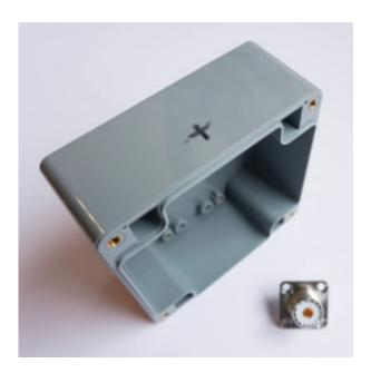
After drilling the 16 mm hole, I placed the chassis part into the hole, to determine the location of the fixing holes. I picked a chassis part where I fix the part with 4 screws, but 2 screws could also work. These holes can be drilled with a 3,5 mm drill.
